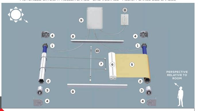
The above system is shown Drive Right, Regular Roll. Brackets shown in Ceiling Mount position.\*
